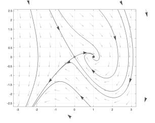
To verify clockwise rotation about the stable focus, observe that to the right of the particular point of equilibrium, i.e., for  $\dot{x} = 0$  and x > 1, it holds that  $\ddot{x} < 0$ , i.e.,  $\dot{x}_2 < 0$  and the vector field points towards decreasing values of  $x_2$ .
